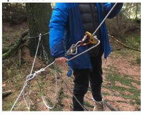
Rigging rope and steel carabiner into maillon on belay cable, then a small fig 8 loop tied about waist height, into which the Petzl Rig, friction krab, and the attachment carabiner for the belayer. Grigri goes and an attachment carabiner for the belayer.
